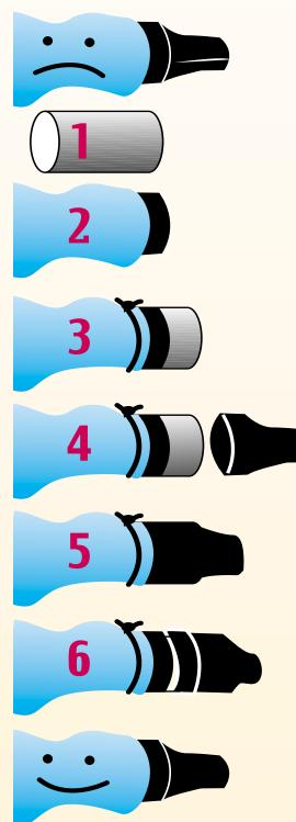
It happens to every drusuit: the unexpected rip of a seal. You can tape them back together with duct tape on both sides at the paddle site. Here's how you install a new one.
